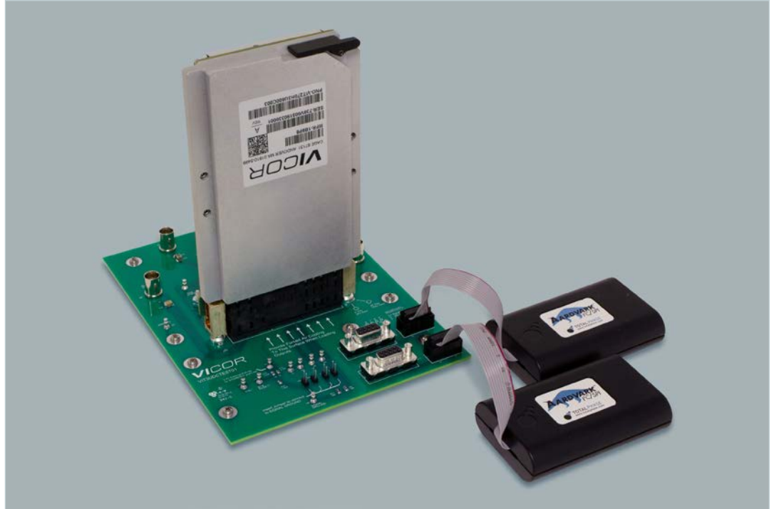
Figure 4 Aardvark™ I 2 C/SPI adapters connected to I2C1 with a VITA62 power supply plugged in
