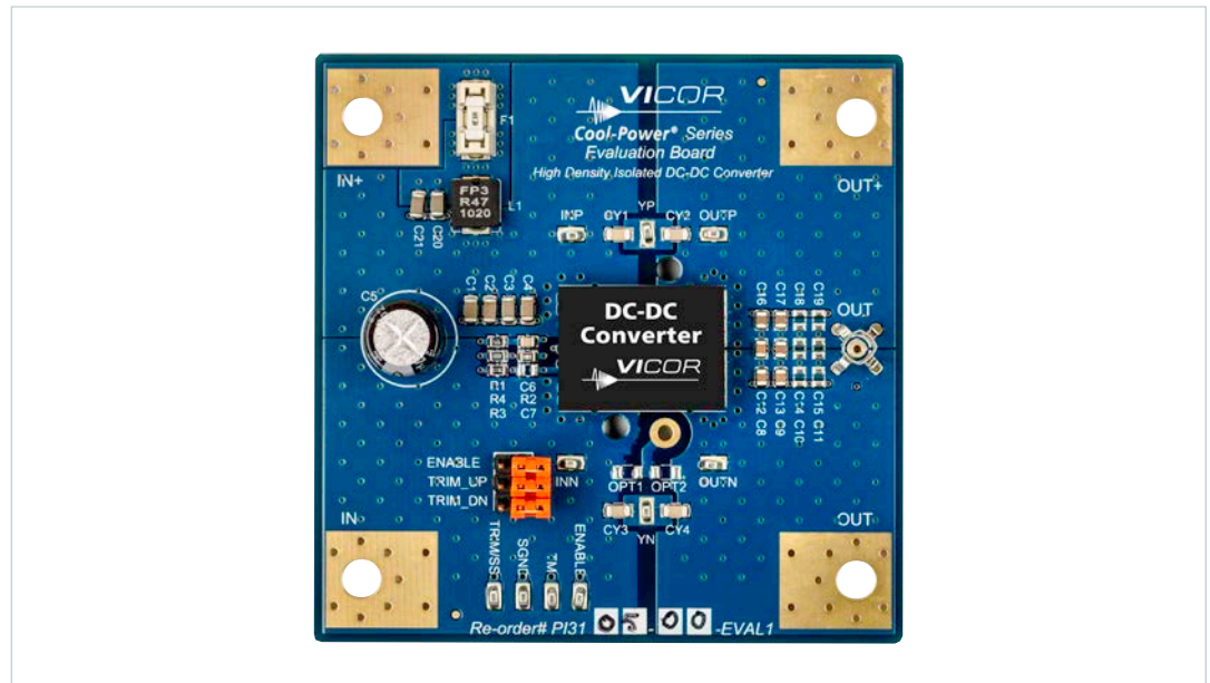
Figure 1 PI31xx-xx-EVAL1 Evaluation Board
