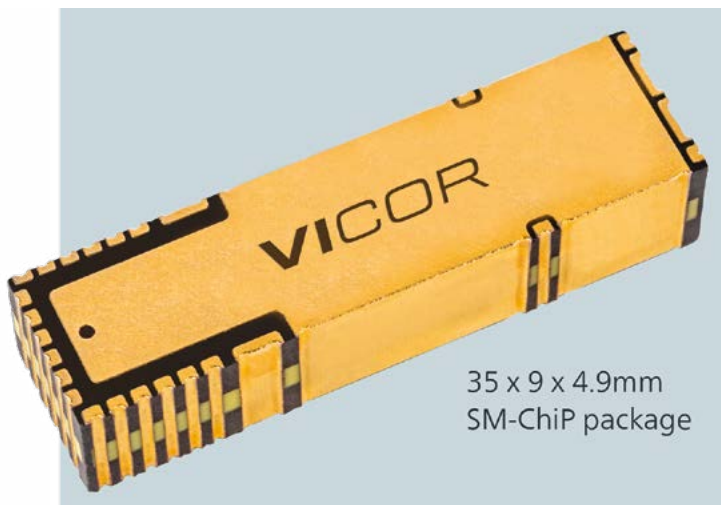
Figure 3: The SM-ChiP package uses laminated construction and direct surface-mount interconnection to the XPU's package substrate and lead frame
