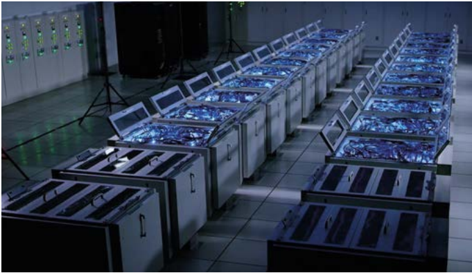
Figure 4: The liquid-cooled Gyoukou ExaScaler/PEZY ZettaScaler-2.2 supercomputer
